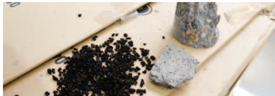
The piece of concrete on the right has been embedded with recycled tires to determine whether they can enhance durability when used in construction.
