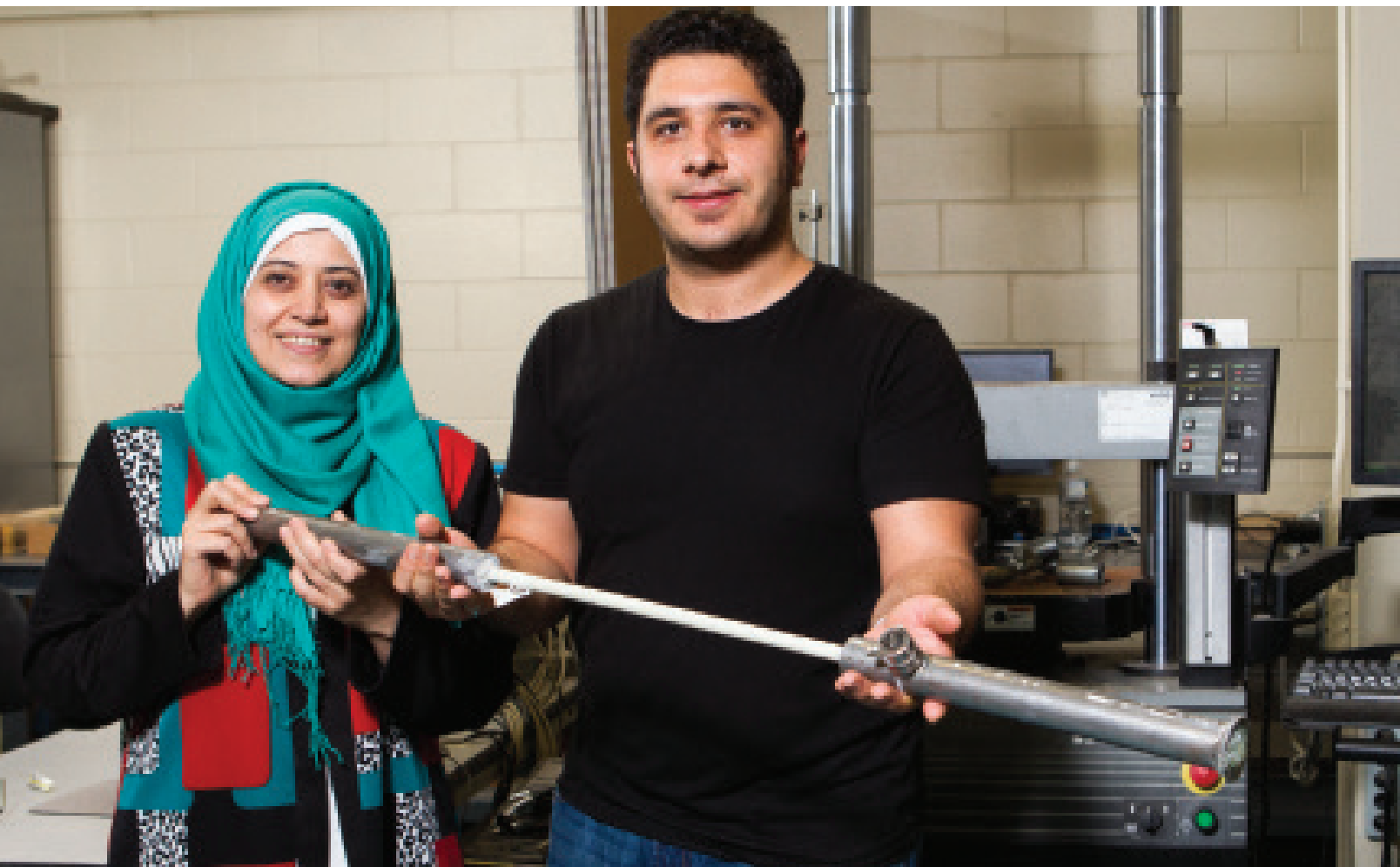
Mohammadhadi Shateri and Maha Ghaib prepare to subject a metal bar made of fibre-reinforced polymers to an acoustic emissions test. Fibre-reinforced polymers resist corrosion and can be used to strengthen construction materials.
