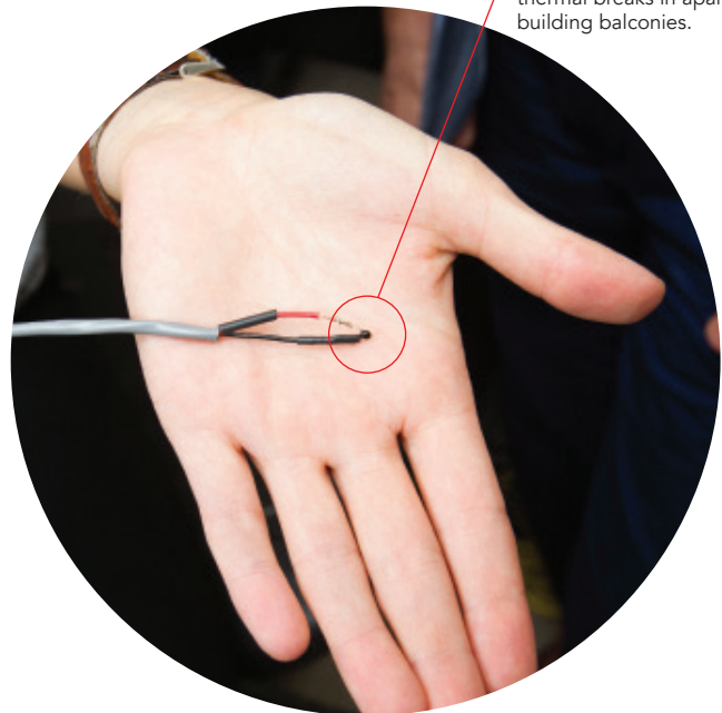
A sensor that is used to test thermal breaks in apartment building balconies.
