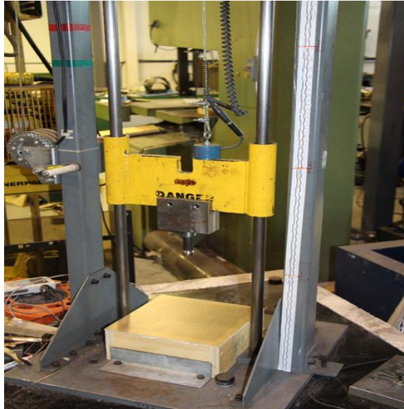
Figure 1. Equipment used in the lab for impact testing 32
